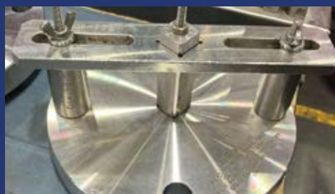
Welding fixture implemented for correct welding alignment
