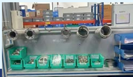
Workbench modification for kitting implementation
